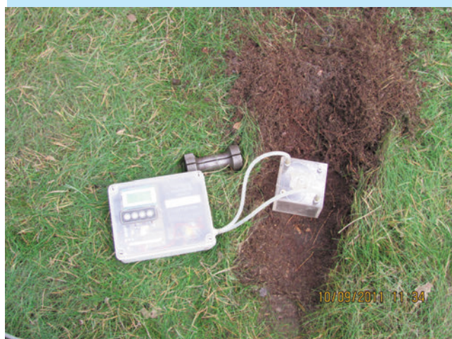
Fig. 17 - An example of field measurement of CO 2 flux in the soil.
